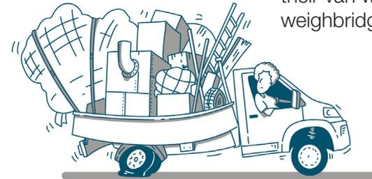
A van has a 'gross vehicle weight (GVW)' or 'maximum authorised mass' (MAM) which can be found on the VIN plate. This is the maximum weight that a van is legally allowed to weigh when loaded. It includes: the van, the fuel, the driver and any passengers and any load being carried. It will be listed in the owner's manual and is normally shown on a manufacturer's plate or sticker fitted to the vehicle. The position of the plate does vary but the most common location is inside the front door panel.
