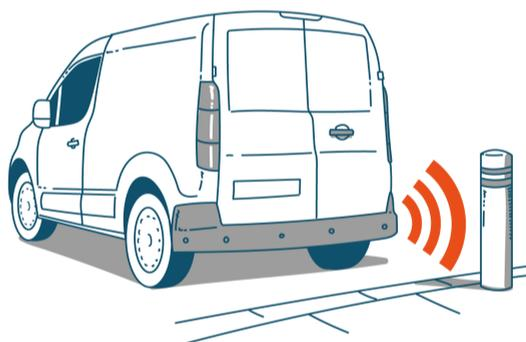
Reversing and parking aids minimise the chances of damage, injury, or prosecution. They can detect obstructions around the vehicle in the driver's blind spot such as bollards, pedestrians and other vehicles.
